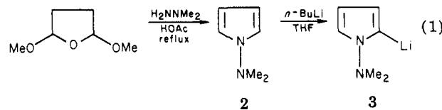
unsym-dimethylhydrazine in acetic acid. Lithiation of 2 (1 M in dry tetrahydrofuran) proceeded smoothly (2 h) with 1.0 equiv of *n*-butyllithium, generating the 2-lithiopyrrole 3. Trapping of 3 with trimethyltin chloride gave 2-(trimethylstannyl)pyrrole 4, bp 68-70 °C (2.0 mmHg),
